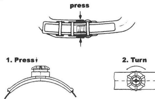
Correct adjustment of the interior ensures that the helmet sits properly.
